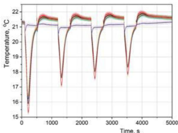
Fig. 3. Degradation of the desorption temperature dip in the repetitive "atmospheric air inflow–pumping out" cycle realized with the sample library shown in Fig. 2.
