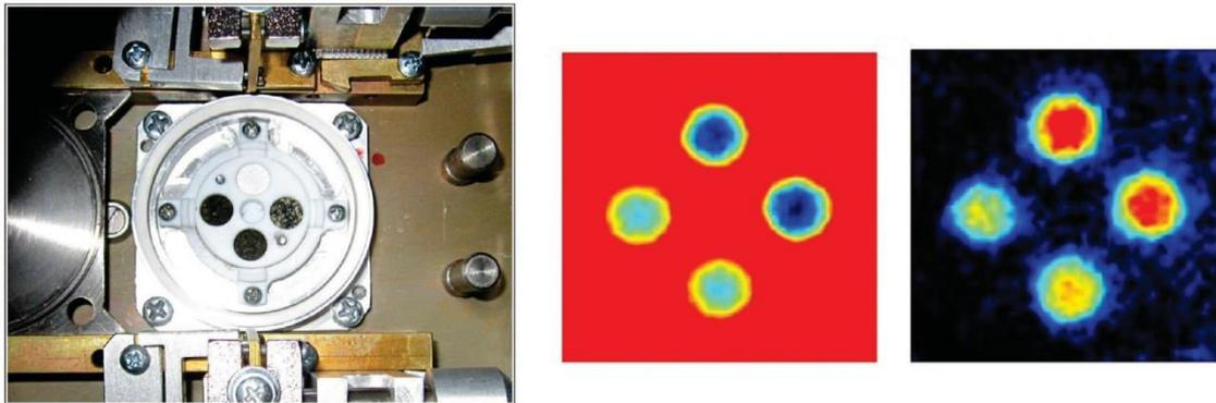
Fig. 2. The library (left) and its two IRT thermograms (right) of highly dispersed samples of aluminosilicates containing different percentages of cobalt and cerium. The library is measured in desorption (left) and adsorption (right) modes, respectively. Despite different colors displayed in a visible-light diapason, these samples, in the infrared spectral range, are identical in their emissivity (this fact is verified experimentally).
